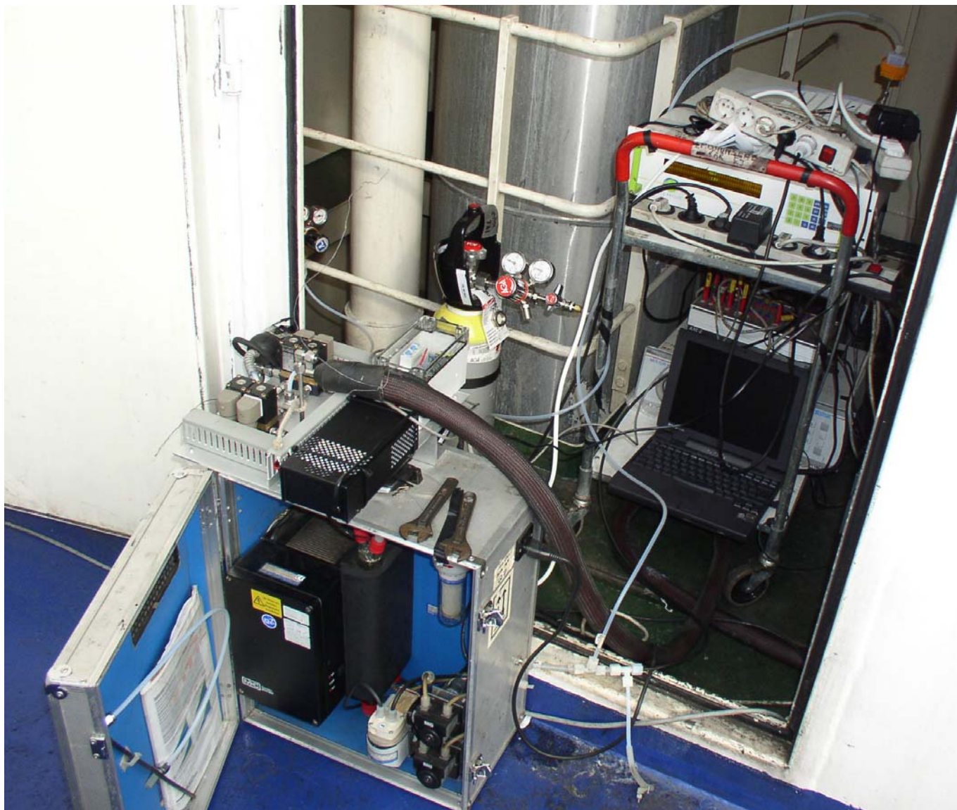
Figure 2. Measurement equipment set-up on board Stena Jutlandica
